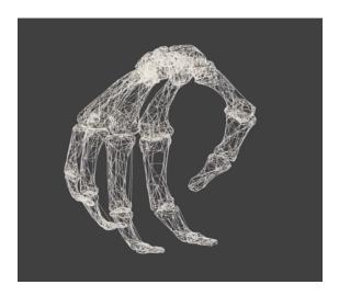
A realtime, 3D rendering program for visualizing hand motion under a robotic exoskeleton. This program communicates over the Internet with the robotic exoskeleton to visualize hand kinematics, as well as torques being applied at each joint. Program was written from scratch with OpenGL and C++.
