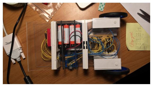
A self-balancing robot built over the summer of 2014. It consists of two DC motors driven by an H-Bridge, 8 AA batteries, an accelerometer, a gyroscope, and an Arduino Micro. Although everything functioned, upright stability was not achieved for more than a few seconds due to the clock speed of the Arduino, and the high torque ratio on the motors which slowed down their response. The structure was constructed with scrap acrylic sheets and cardboard cutouts.
